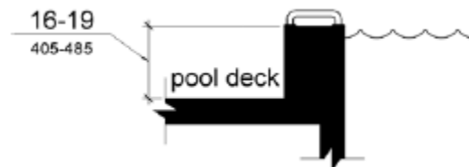
Figure 1009.4.2 Transfer Wall Height
